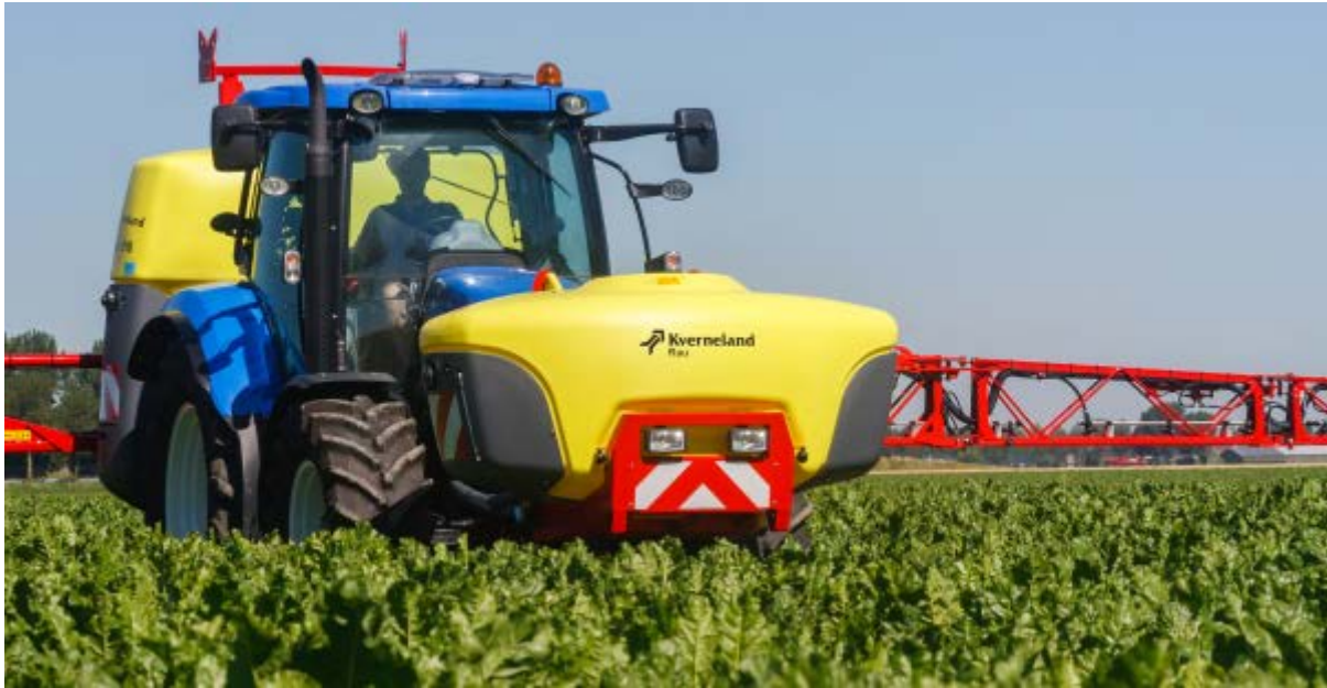
Kverneland Rau iXtra Front Tank in combination with the iXter mounted sprayer
