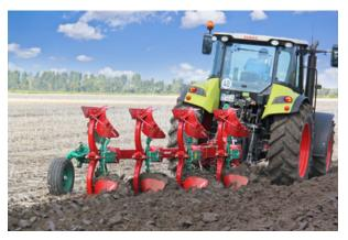
70/75cm underbeam clearance for the 150 S Variomat (80 cm for the 150 B Variomat) and 85/100cm interbody clearance for best performance in various soils and surface conditions.
